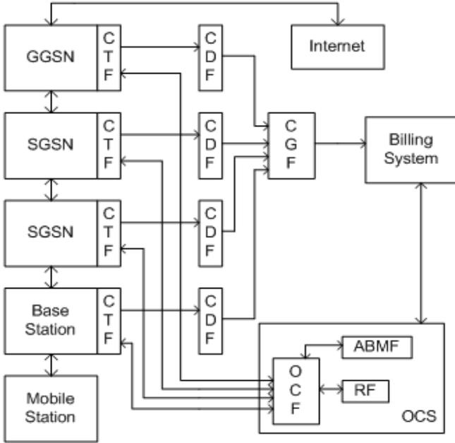
Fig. 1. UMTS charging architecture
