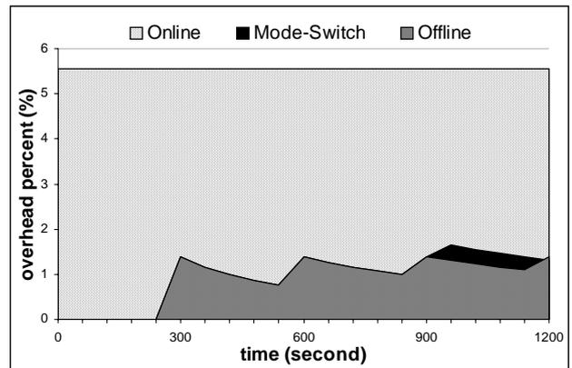
Figure 4. Percentage of the charging overhead during the service
