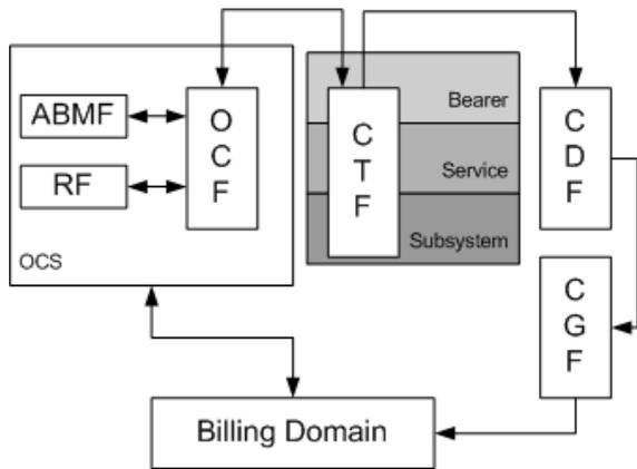
Figure 2. Functional architecture of the offline and online charging
