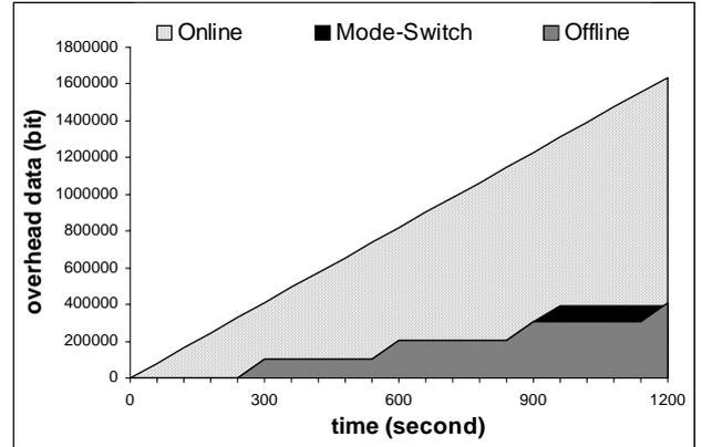
Figure 3. Size of the charging overhead during the service
