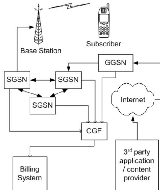
Figure 1. Packet-switched charging architecture
